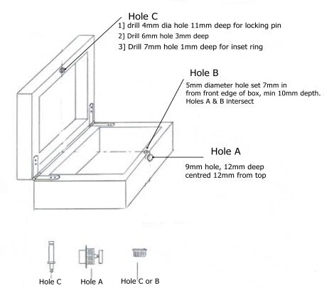
For best results use a drill press. Min wall thickness 12.5mm The Inset ring may be used on either holes B or C, for fitting to hole B follow steps 2 & 3 marked on Hole C. Always fit and align box hinges before fitting catch. Fit main button in hole A first, the locking pin can be located by locking into the main button and gently pressing the lid to make a fitting mark (depending on wood hardness). These are fitting guides only and some minor adjustment may be needed for a final quality fit.
